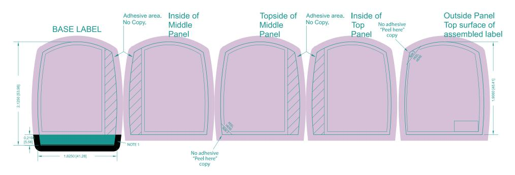
Note 1: Lot and Exp. code will be laser printed. This area must be dark color to provide sufficient contrast to white base label. No copy or varnish area.
