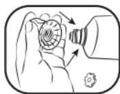
4. Screw the applicator cap back on the tube
