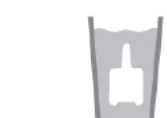
If spray nozzle is clogged, soak in warm water. Then repeat steps 2 and 3.
